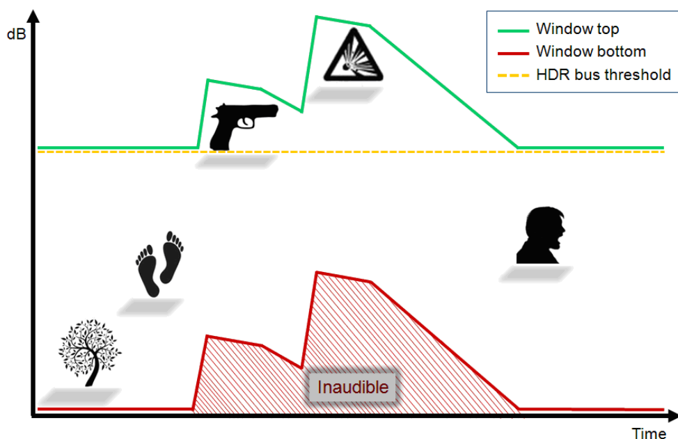
Figure 29.7. HDR overview, as seen on the input side of the system
