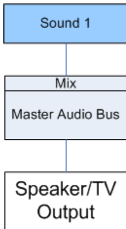
Figure 29.2. Simple example of a sound going to the main output
